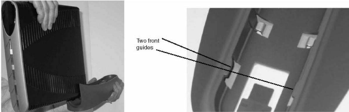
Slide the base in from the rear of the unit, by using the locating guides.
