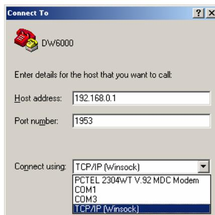
Select connect using TCP/IP, and enter 192.168.0.1, port 1953
