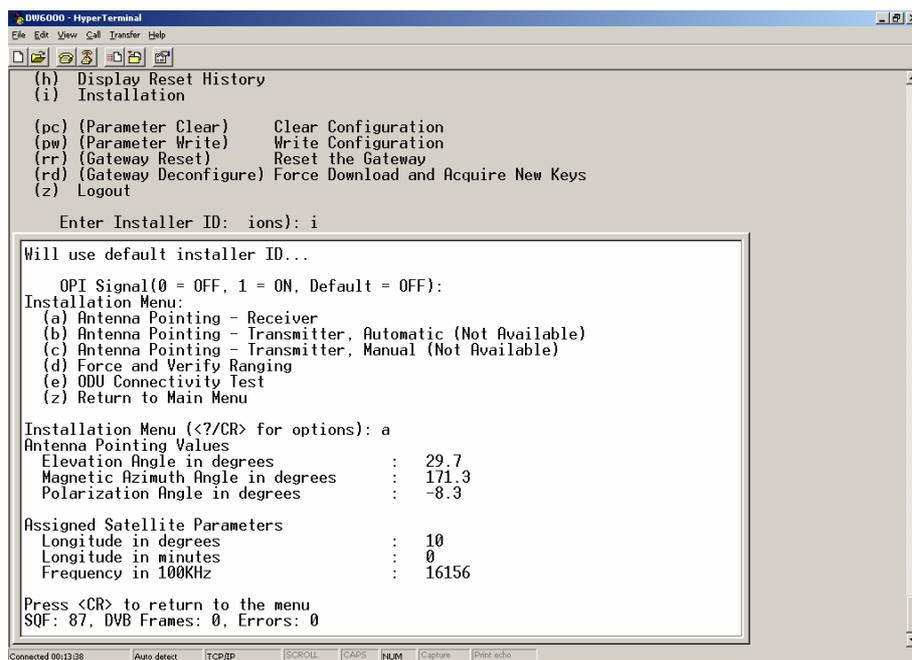
Fine tune the antenna with the values for Elevation, Azimuth and Polarization angles displayed on your screen.
