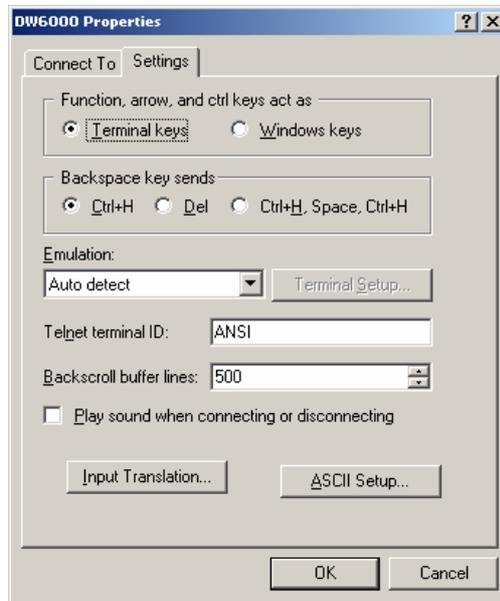
Ensure the settings are as shown above, then select ASCII setup
